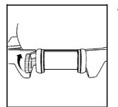
Unlatch the seat from the floor by lifting the lever located next to the carrying handle on the rear of the seat near the bottom.
